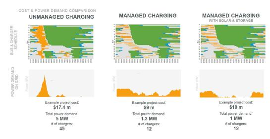
Comparing unmanaged, managed on grid only, and managed with solar and battery storage for power consumption and costs.
