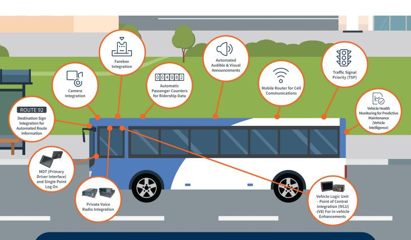
Vontas Intelligent Transportation Systems make each journey safe, reliable, smart, and connected through the integration of various on-board devices that accurately track the bus along its route, enable real-time voice and data communication, and keep passengers fully informed.
